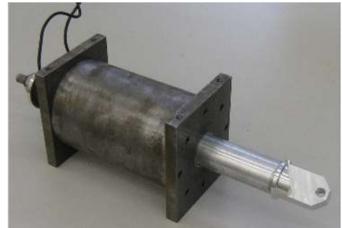
Fig. 7. Prototype of the final design of the actuator.
