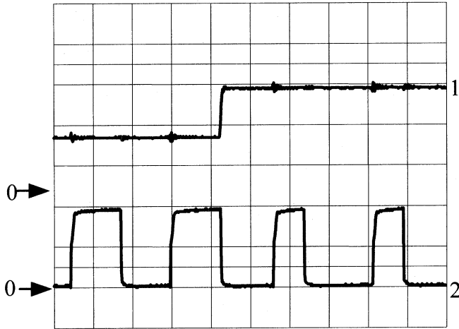
Fig. 11. Main switch duty ratio response to V_d steps from 35 V up to 55 V. f_s = 200 kHz. Traces: 1-input voltage (20 V/div.); 2-feed-forward gating command (5 V/div.). Timing-2 \mu s/div.
