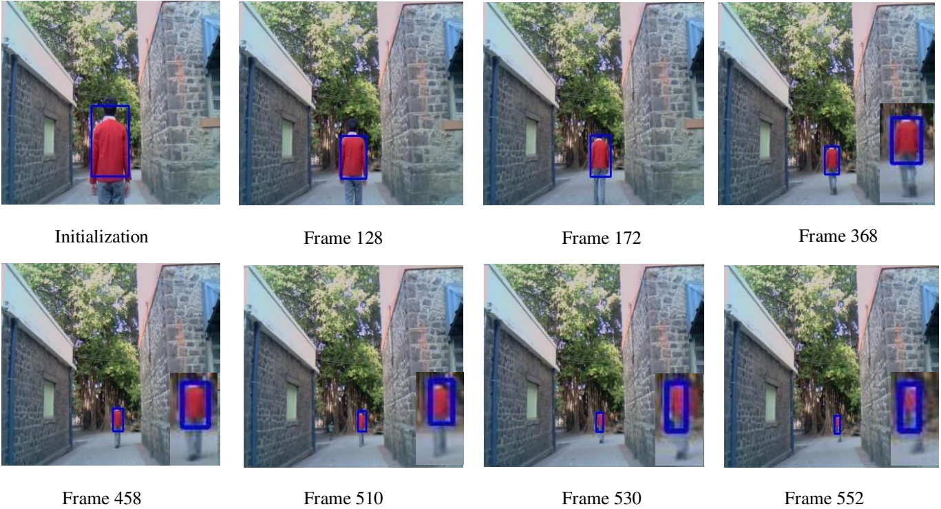
Figure 2. The performance of our tracker from a real life outdoor sequence. Tracking accuracy is maintained as the target undergoes rapid changes in scale as it can be seen in the inset from frame 368 onwards.
