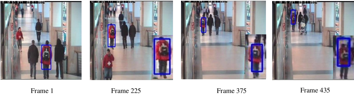
Figure 3. Demonstration of scale adaptive tracking using the CAVIAR dataset test sequence ThreePastShop2cor.mpeg. Frame 1 is offset from the CAVIAR video by 390 frames. A magnified view in inset from frame 225 onwards
