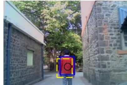
Figure1(c). Selection of the localization circle S_n in black. C_n shown in blue and one of the candidates for R_n in dashed yellow.
