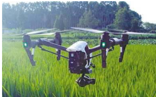
Figure 10. Hyperspectral sensor on-board a DJI T600 unmanned aerial vehicle (UAV).
