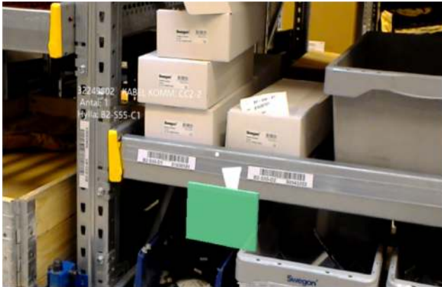
FIGURE 5. The AR interface with visual aid for the order picking in HoloLens.
