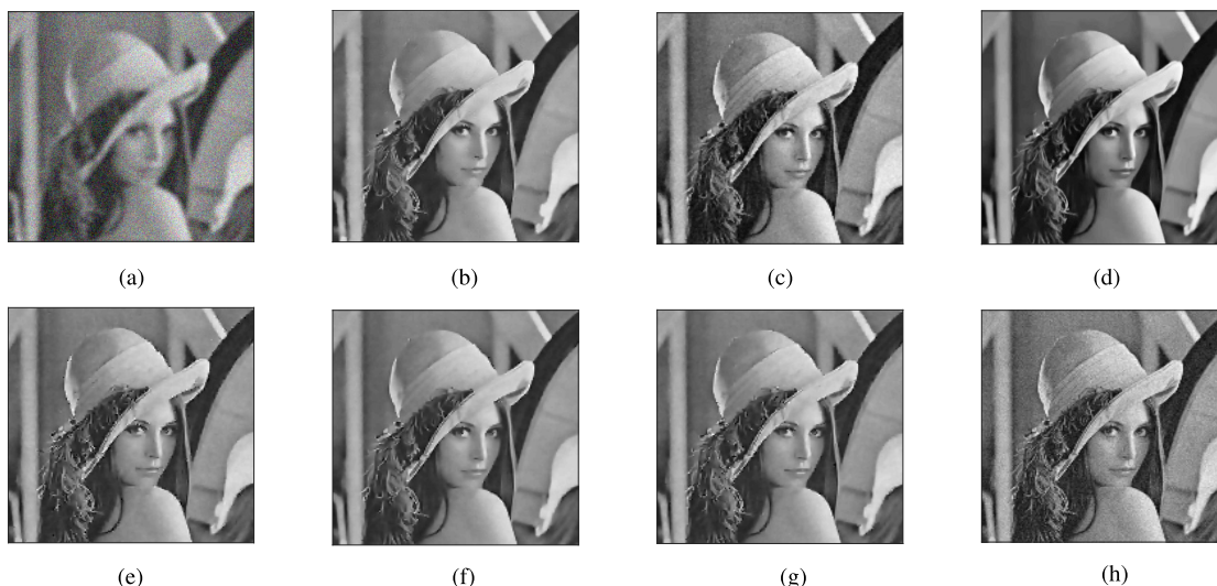
FIGURE 12. Denoising results for the image Lena degraded due to Gauss blur ( G ) and Gaussian noise having standard deviation of 20 (a) Noisy image (b) R-NL, PSNR (SSIM) = 29.34(0.831); (c) Cuesta, PSNR (SSIM) = 27.04(0.753); (d) Ada-Reg, PSNR (SSIM) = 30.12(0.813); (e) FTV-PA, PSNR (SSIM) = 27.69(0.752); (f) OLGS, PSNR(SSIM) = 30.27(0.832); (g) FFAD, PSNR(SSIM) = 29.43(0.831) (h) HF-OLGS, PSNR(SSIM) = 31.12(0.874). (a) Noisy image.
