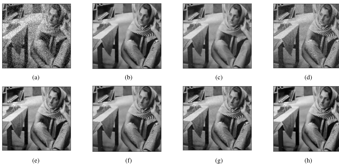
FIGURE 13. Denoising results for the image Barbara degraded due to Gauss blur ( G ) and Gaussian noise having standard deviation of 30 (a) Noisy image (b) R-NL, PSNR (SSIM) = 28.96(0.761); (c) Cuesta, PSNR (SSIM) = 26.80(0.749); (d) Ada-Reg, PSNR (SSIM) = 28.78(0.731); (e) FTV-PA, PSNR (SSIM) = 25.31(0.753); (f) OLGS, PSNR(SSIM) = 29.31(0.841); (g) FFAD, PSNR(SSIM) = 27.92(0.776) (h) HF-OLGS, PSNR(SSIM) = 29.37(0.852). (a) Noisy image.
