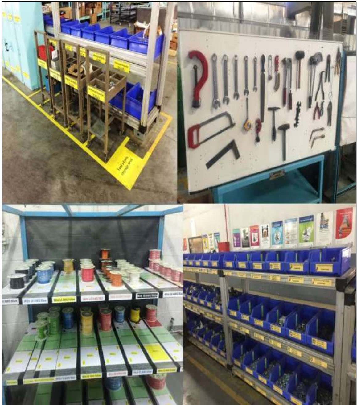
Figure 4-13: Sample of 5S technique at Al Salem Johnson Controls
