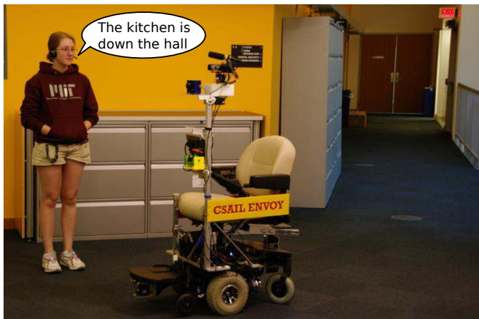
Figure 1: A user gives a tour to a robotic wheelchair designed to assist residents in a long-term care facility.
