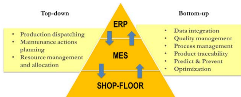
Figure 6 MES integration with ERP and the information tools used at the shop-floor level (see online version for colours)
