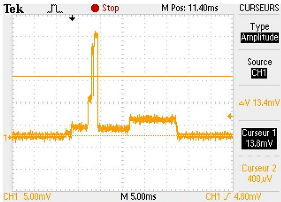
Figure 5 Measured current for the EZ430 platform.
