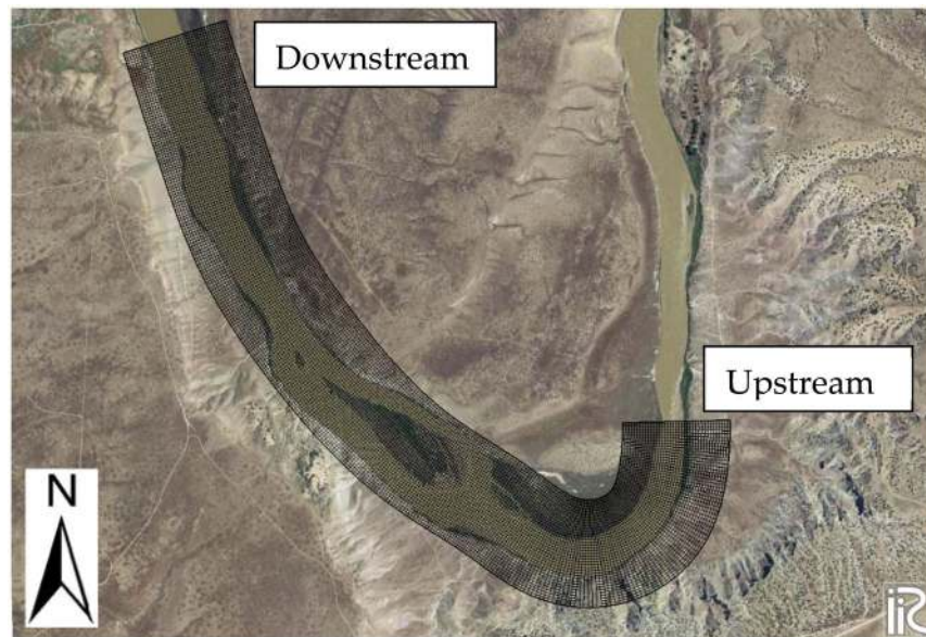
Figure 2. Meshed geographic data shows the computational domain in the iRIC. The grid cells are 5 (x) × 5 (y) meters. Figure was created in iRIC version 3.0.18, revision 6257 ( https://i-ric.org/en/ ).
