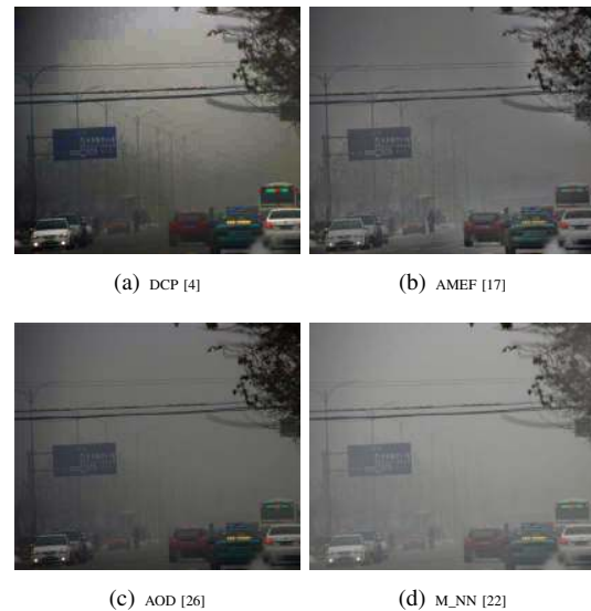
FIGURE 10. Task-driven comparison: either haze is not removed completely or blocking artifacts are injected in the de-hazed image.
