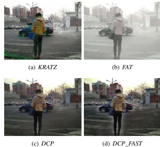
FIGURE 2. (top) - Example result from Kratz et al. [15] and Fattal [5], clear color shift artifacts are visible. (bottom) - Quality comparison among the DCP [4] technique and its fast version DCP\_F . Visible halos artifacts, around objects, are produced with the fast version.
