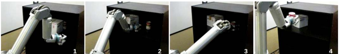
Fig. 7. An example plan to retrieve a can hidden behind a large box on a shelf. The pick-and-place planner fails to find a plan in this scene. But pushing planner finds the presented plan. Planning time is 51.2 sec.
