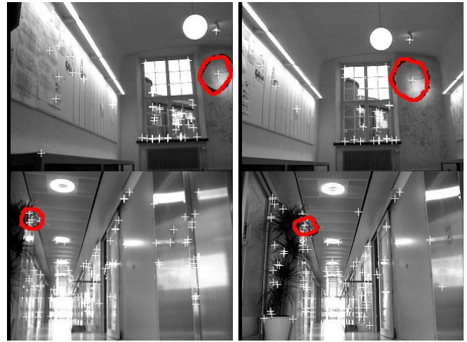
Fig. 7. Two other loop closing situations, one from the atrium area and one from an office type environment. After returning to an area the robot successfully matches landmarks from the previous time it was there. The circles show the matched pair of features. The right hand side shows the image from the data base.
