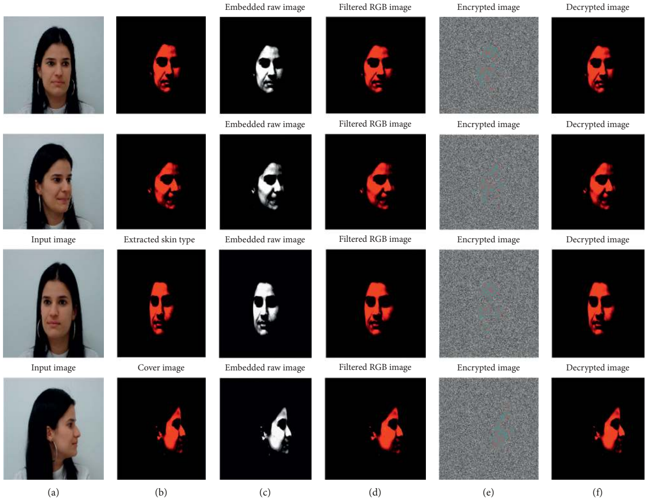
FIGURE 5: Simulation results of the embedding scheme using V-DWT and Lagrange interpolation encryption using different imaging conditions and different poses of an input image. (a) Original images (image 1 to image 4), (b) high-intensity layer as the cover image, (c) embedded raw image, (d) color space converted stego image, (e) encrypted image, and (f) decrypted output image.
