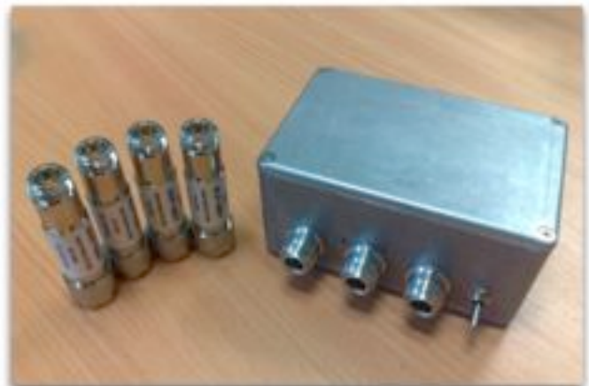
Figure 3. A Low-power 3-channel detector with externally mounted band filters.
