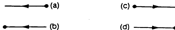
Figure 1. Parts of diagrams representing the (a) creation of an electron, (b) annihilation of an electron, (c) annihilation of a hole, and (d) creation of a hole.
