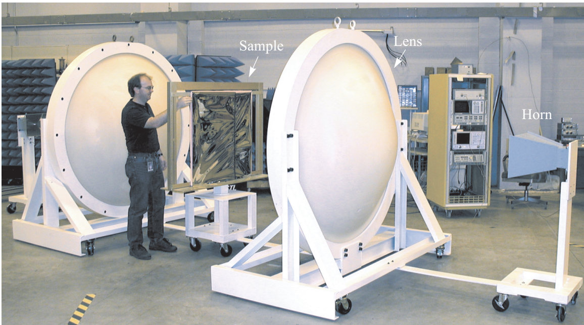
Figure 1.9: Photograph of a focused-beam system designed to make material measurements for frequencies as low as 800 MHz. Image credit: Dr. John Schultz and STL/GTRI.
