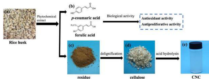
Figure 5. A flowchart of rice husk full utilization. (a) the photo of rice husk; (b) the main phenolic compounds in rice husk; (c) the picture of residue after phytochemical extraction; (d) the cellulose gained after delignification; (e) the CNC prepared by acid hydrolysis from cellulose of rice husk.
