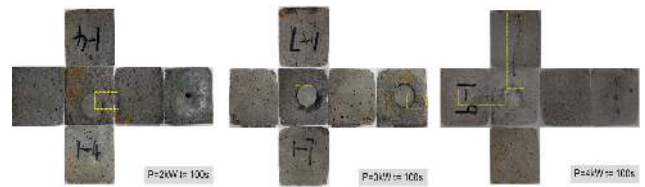
FIGURE 7. Cracks formation in mortar-granite sample under microwave treatment.
