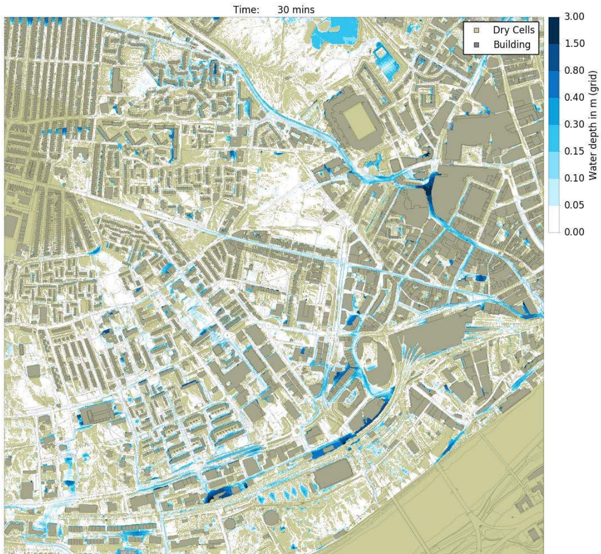
897 898 Fig. 14. Water depths over the whole modelled domain of 4km 2 at the end of a 30 minutes rainfall 899 event with 100 years return period - current situation 900
