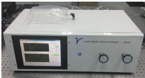
FIG. 1. Photograph of the fully integrated, standalone, portable breath acetone analyzer.
