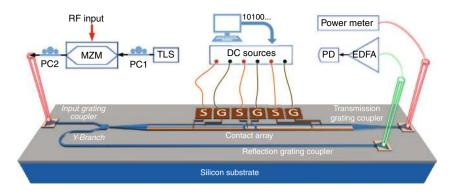
**Fig. 4** Schematic view of a programmable microwave signal processor. The experimental set-up consists of a tunable laser source (TLS), a polarization controller (PC), a Mach-Zehnder modulator (MZM), an erbium-doped fiber amplifier (EDFA), and a photodetector (PD)
