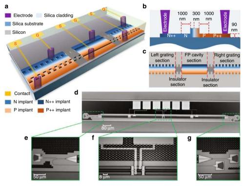
Fig. 2 The designed reconfigurable grating. a Perspective view of the grating on a silicon chip. b Cross-sectional view of the grating rib waveguide. c Topview of the grating. d-g Microscope camera images of the fabricated grating, the input grating coupler and compact Y-branch, the FP cavity section, and the transmission and reflection grating couplers
