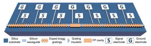
**Fig. 1** Schematic view of reconfigurable grating. The grating consists of multiple series-connected uniform Bragg grating sections and an FP cavity section in the center of the grating. Each uniform Bragg grating section incorporates an independent lateral PN junction, and between two neighboring sections there is an un-doped grating to function as an insulator. A pair of electrodes (Signal and Ground) are connected to each independent PN junction
