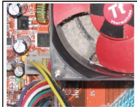
Figure 4: Heat sink fouling in a conventional CPU cooler. The finned heat sink, which is stationary, cannot be seen because it's completely covered in dust. The fan blades, which rotate at several thousand rpm, are nearly dust-free despite operating in the same environment.
