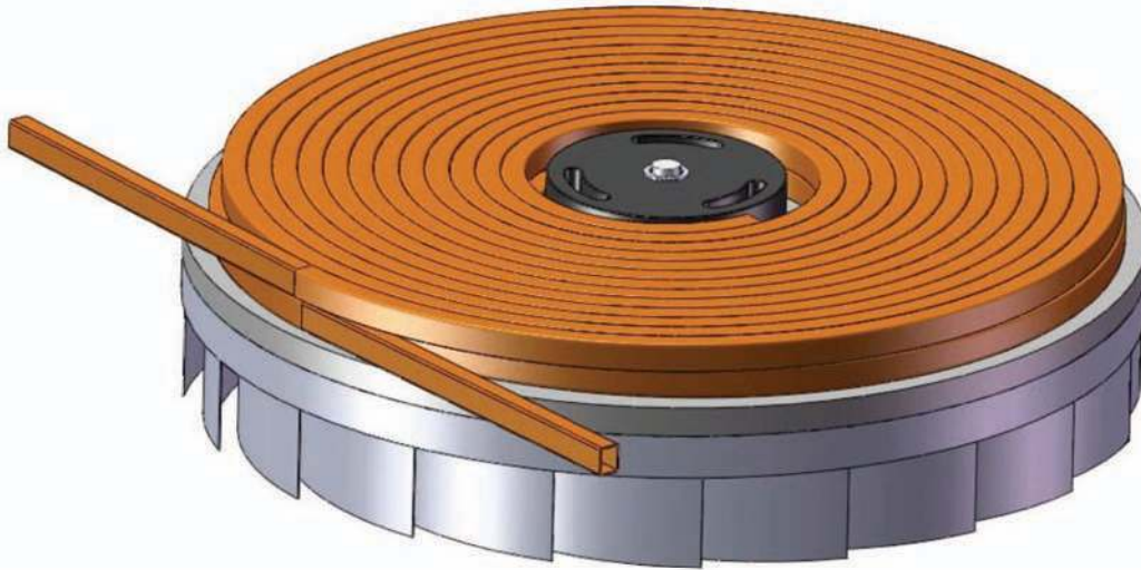
Figure 8: Schematic drawing showing application of air bearing heat exchanger concept to an air conditioner condenser. Such a unit can be made extremely compact compared to a traditional fan-plus-serpentine-finned-tube architecture, and fouling of the outer surface of the soldered copper tubing assembly has no effect on condenser performance. A second identical air bearing cooler (not shown) can be fused to the opposing face of the soldered copper tubing assembly to lower the thermal resistance of the heat exchanger by an additional factor of 2 if desired. An air conditioner evaporator unit can be implemented in an analogous structure. In the case of the air conditioner evaporator, it is also possible to enclose the heat-sink-impeller assembly in a plenum, such that it also serves to circulate air through the HVAC air duct system.
