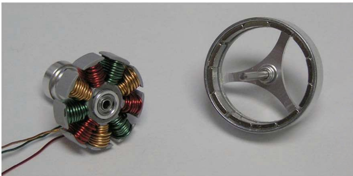
Figure 15: At left, 9-pole, 3-phase internal rotor. At right, 12-pole permanent magnet external rotor.
