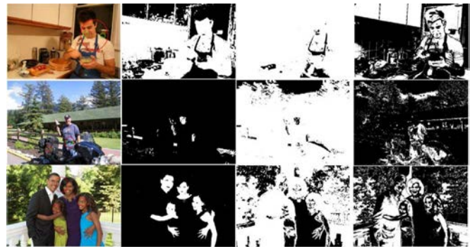
Fig. 13. Column from left to right represent original images, skin detection using [19], [32], and our proposed method, respectively.
