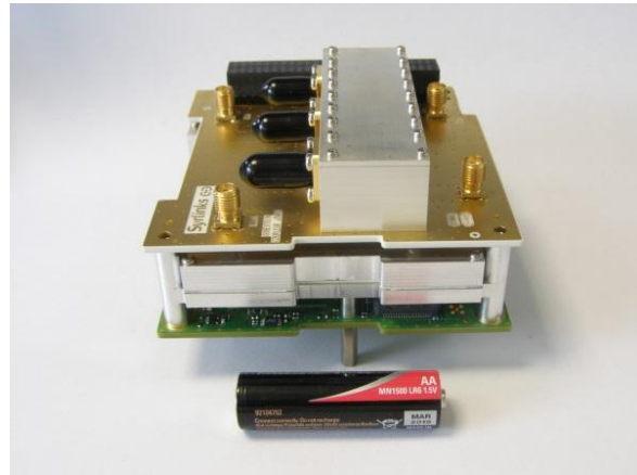
Figure 1 : EWC31 S band TT&C/ISL with 1 first diplexer configuration and integrated coupler
