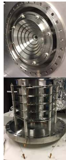
Figure 5: Left: technical drawing of the new setup. The gas cell (left volume) hosts from left to right the entrance window (blue), the cage (red), the funnel (green), the filament (cyan) and the nozzle (yellow). The gas jet chamber has a view port for the laser and a curved RFQ (purple) for ion extraction. For details see text. Right: Photographs of the funnel (top picture) and the cage structure (bottom picture) before installation.
