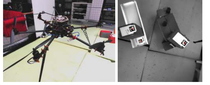
Fig. 4: On the left, a picture of the fully-actuated UAV used in the experimental validation, while on the right a picture taken from the onboard camera about the feature detection.
