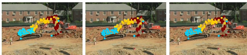
Fig. 6. A sequence of a bulldozer with its upper-arm and forearm moving articulately around some axis. The color of a dot, red, blue or yellow, shows the segmentation result. There are 4 misclassification errors. Two are the yellow dots on the forearm and two are the red dots on the upper-arm. All of them are near the axis connecting both arms. Besides these, there are several outliers in the trajectories and they are clustered to one of the segments.
