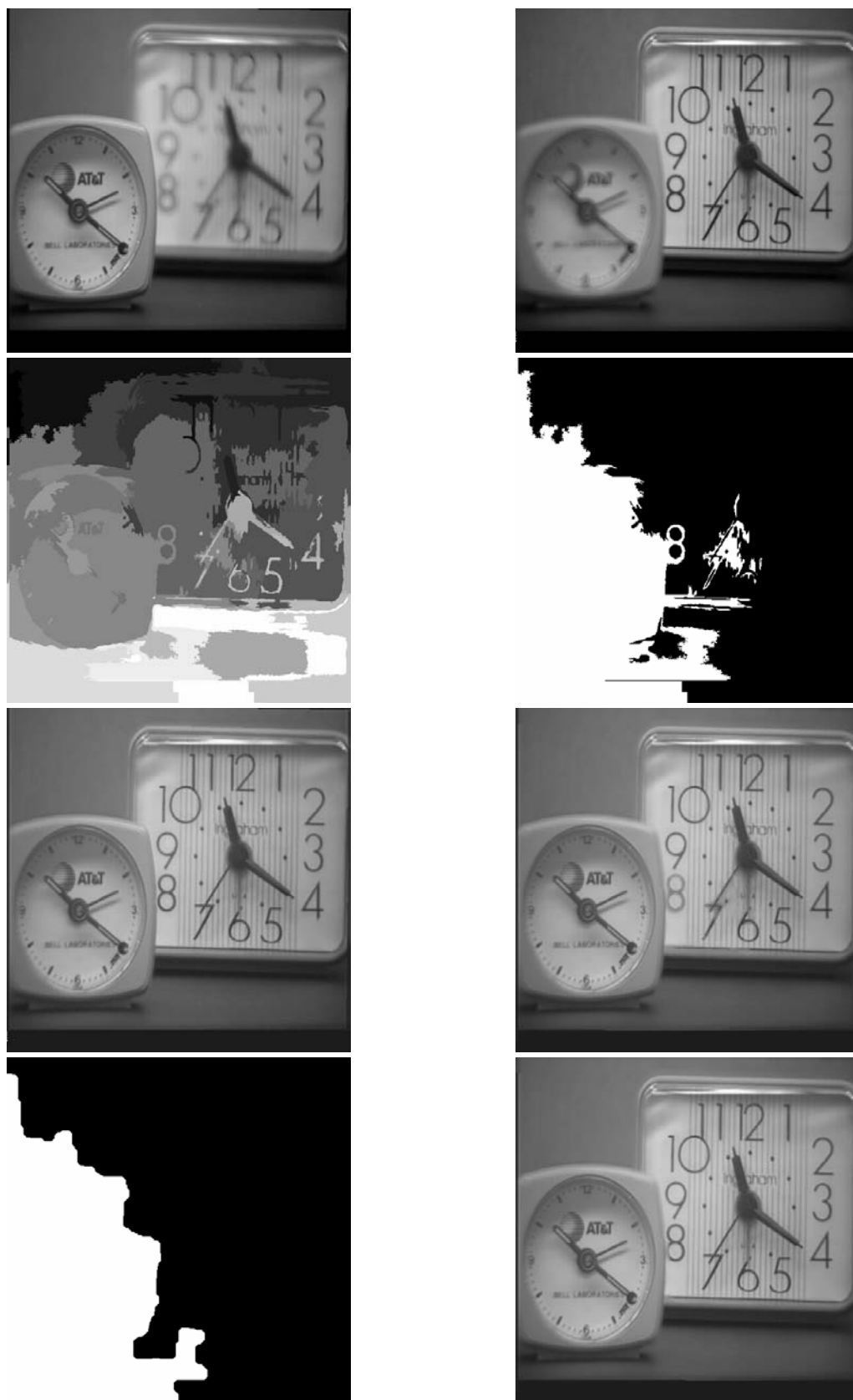
Figure 31: Example 2. Top: multi-focus test images; second row: 1st level of segmentation (left) and decision map (right); third row: fused images with pixel-based (left) and region-based (right) approach; bottom: filtered decision map (left) and corresponding fused image.
