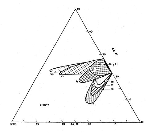
Fig. 1 - Ni<sub>3</sub>Al solid - solution field at approximately 2100°F for various ternary alloys. After Guard and Westbrook (3).
