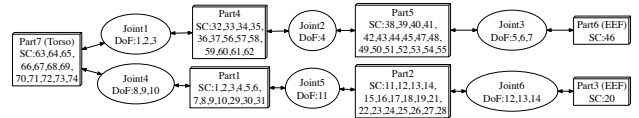
Fig. 4. Structural exploration result: kinematic tree HRP-2's upper body, visualizing the dependencies of joints (featuring one or multiple DoFs) and body parts (featuring one or multiple SCs) towards the torso (root of tree)
