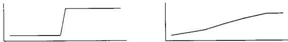
Fig. 5. When p = 1 , any monotone functions which are equal at the beginning and end must have the same total cost. Therefore, both the sharp edge and the smooth edge have the same cost.
