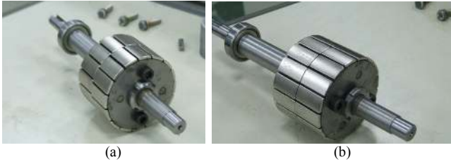
Fig. 17 Features of the rotors (magnets included): (a) with 3.75^\circ\text{M} skew (Case 1); (b) without skew (Case 2). The skew for (a) is a step skew which uses two axial rotor sections with an angular offset.
