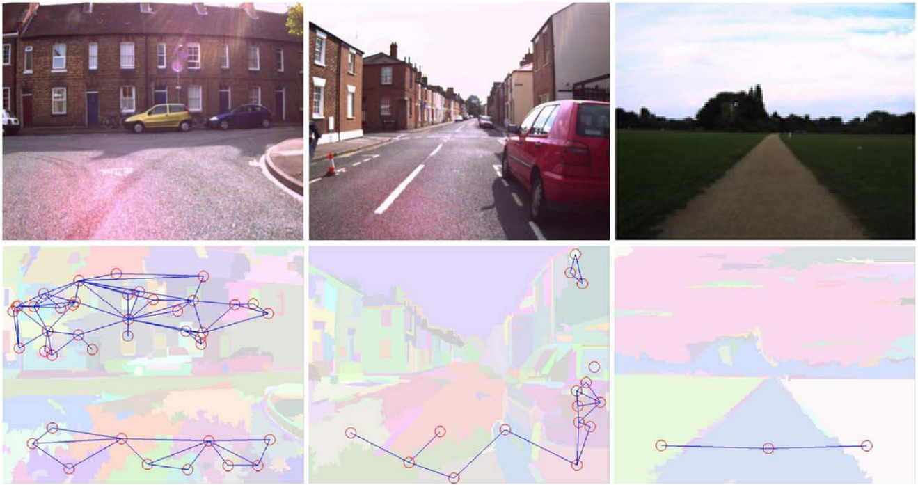
Fig. 5 Typical graphs extracted from urban scenes as recorded by our mobile robot. Top : the original scenes. Bottom : the corresponding segmented images with the extracted graph overlaid. Circles indicate
