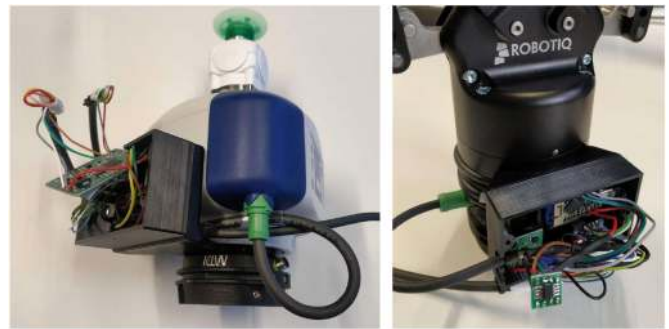
FIGURE 9. Custom Wi-Fi OPC UA tool adapter based on the TinyPICO microcontroller board running FreeRTOS: Schmalz ECBPi (left) and Robotiq 2F-85 (right). The only external connection required is a 24V power supply provided through the tool changer.
