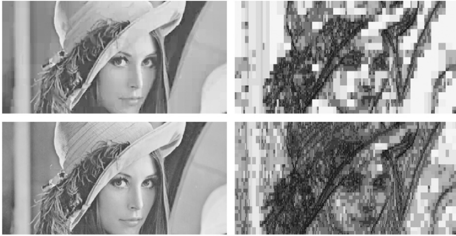
Fig. 2. Image Lena 512 \times 512 coded with MMP at 0.128 bpp (top) and 1.125 bpp (bottom), with the respective generated filter support maps using \tau = 32 .
