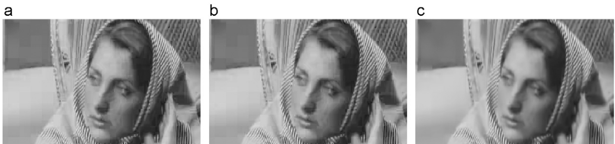
Fig. 6. A detail of image Barbara 512 \times 512 , encoded with MMP at 0.316 bpp. (a) No deblocking 30.18 dB. (b) Method from [22] 30.18 dB (+0.00 dB). (c) Proposed method 30.31 dB (+0.13 dB).
