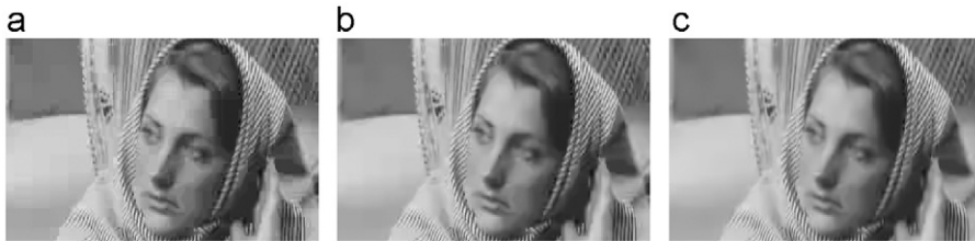
Fig. 8. A detail of image Barbara 512 \times 512 , encoded with H.264/AVC at 0.321 bpp. (a) In-loop deblocking [9] disabled 29.72 dB; (b) In-loop deblocking [9] enabled 29.87 dB (+0.15 dB). (c) Proposed method 29.84 dB (+0.12 dB).
