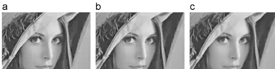
Fig. 5. A detail of image Lena 512 \times 512 , encoded with MMP at 0.128 bpp. (a) No deblocking 31.38 dB. (b) Method from [22] 31.49 dB (+0.11 dB). (c) Proposed method 31.67 dB (+0.29 dB).
