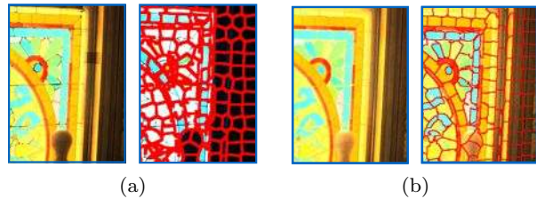
Fig. 11 Superpixel segmentation of (a) HDR image and (b) LDR image.
