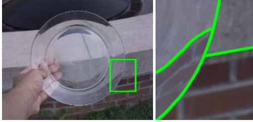
Figure 2. Comparing two background regions to their glass-covered versions we expect to get a high discrepancy value. We will get low values when comparing the two background regions, the two glass regions, and the glass regions to the background region that does not correspond to it. This will allow for two possible segmentations, the correct glass/background segmentation and another with one glass region and the background that is not its own.
