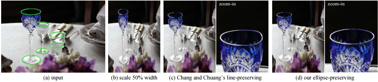
Figure 11. Images resizing with ellipse preservation. (a) Input image and user-marked ellipses. (b) Uniform scaling. (c) Chang and Chuang’s [7] line-preserving retargeting. (d) Our result with ellipse preservation.
