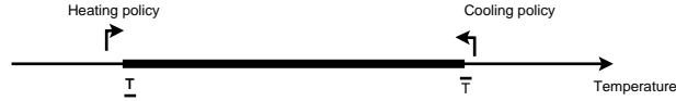
Figure 1: The single dimensional temperature regulation example. If the temperature is higher than \bar{T} the control policy is to cool, and if the temperature is lower than T the control policy is to heat.
