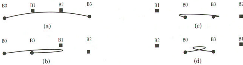
Fig. 10. Four cases for collinear cubics. Assume the control points converge to the horizontal line defined by the two endpoints. (a) Case (1), monotonic motion of t ; (b) Case (2), one fold; t changes direction once; (c) Case (3), two folds; t changes direction twice; (d) Case (4), two folds; t changes direction three times.
