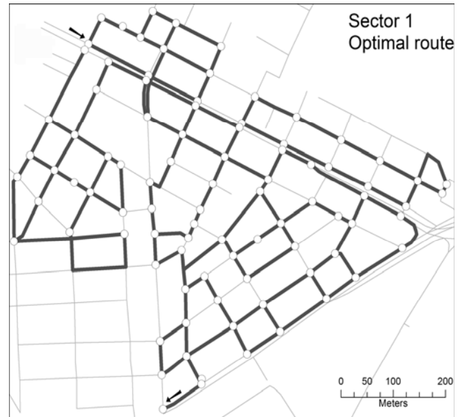
Fig. 5: Optimal waste collection vehicle route.
