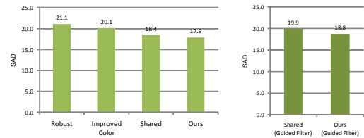
Figure 10. Quantitative comparisons on average SAD error of \alpha , with post-processing. Left: post-processing via the matting Laplacian. Right: post-processing via guided filter.
