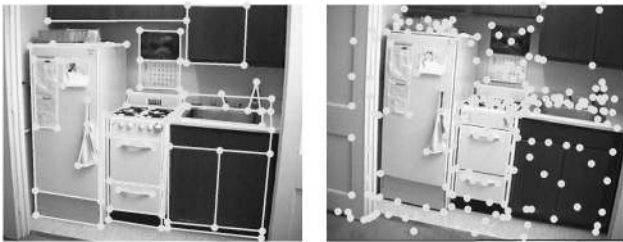
Fig. 9. Two images— 480 \times 512 pixels, 256 gray levels—from the Kitchen sequence with spurious features. Wireframe is for better perception only.
