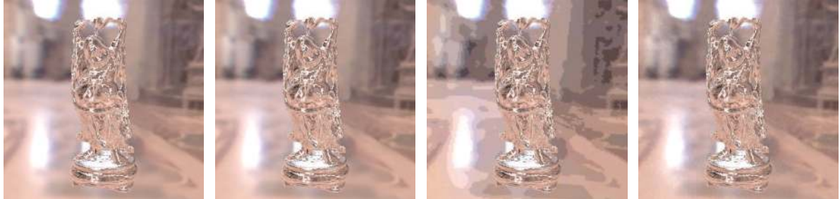
Figure 1: A simple real-time application showing Happy Buddha with emphasis on texturing operations for timing: on the left Ground truth HDR texture was encoded using 32bit floating point for each channel (96 bpp). On the center left RGBE encoding (32 bpp). On the center right Wang et al. [28] (16 bpp), note that in this case the splitting axis between LDR and HDR image minimizes RMSE error but appearance presents noticeable quantization artifacts. On the right our method using residuals (8 bpp).
