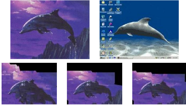
Figure 6. We match the top-left image to the top-right image with different value of the crossing constant \mu (on the bottom). From left to right, \mu = 0, .5 and 1.5 .
