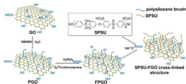
Scheme 2 Preparation procedure of SPSU/FPGO cross-linked membrane.
