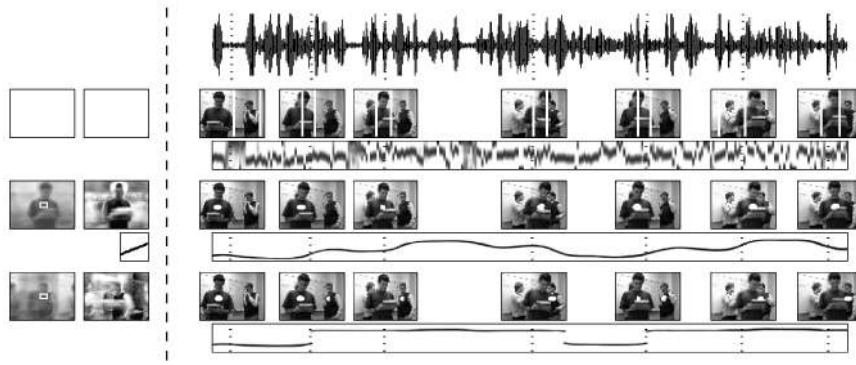
Fig. 4. Tracking results for the audio only (first row), audio-video (second row), and video only (third row) models. Each row consists of the inference for \ell_x (bottom), and selected frames from the video sequence (top), positioned in time according to the vertical dotted lines. Note that while the subject moves horizontally, the bottom row of each plot depicts \ell_x inference on its vertical axis for clarity. The area enclosed by the white dots, or between the white lines in the case of the audio only model (first row), represents the region(s) occupying the overwhelming majority of the probability mass for the inferred object location.
