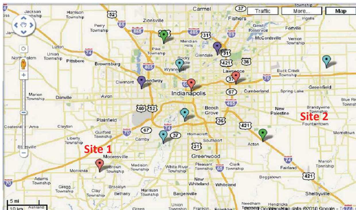
Figure G-1. General map of the Indianapolis area showing the locations of idealized (STILT back trajectory chosen) tower locations (colored push pins). Site 1, located in Mooresville, is upwind and will provide a 'local background' site. Site 2, located on the east side of the city, will capture the urban plume when the wind is aligned in the predominant vector (a northwest wind).
